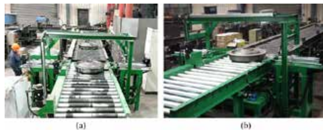
Fig. 4. High-speed rail automatic three-dimensional measurement line (Chen Xu., 2019)
