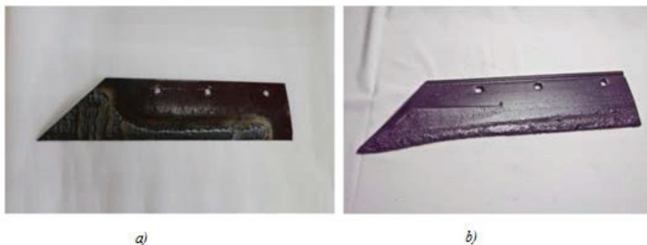
Fig. 6. Plowshares for the ПЛН-3-35 plow: a – experimental plowshare for sandy loam soils; b – series-produced plowshare
