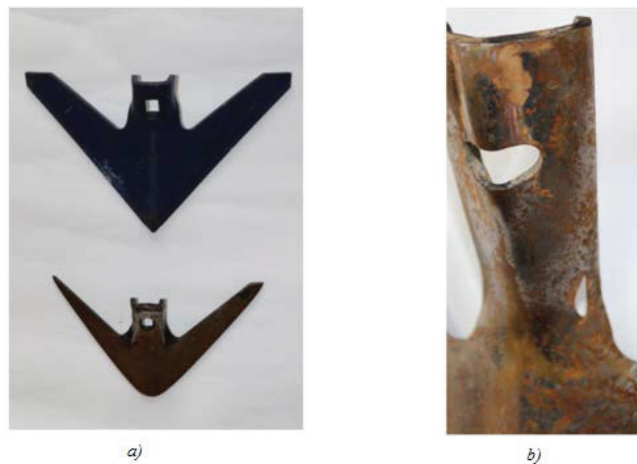
Fig. 9. Reasons for the loss of the working condition of the center hoes: a – plow-point and wing wear in width (on the example of a new and worn hoe); b – wear of the fastening part
