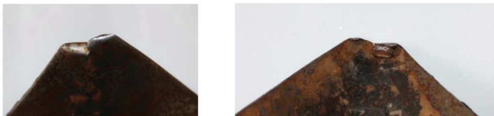
Fig. 10. Cultivator plow-point after bending and breaking off
