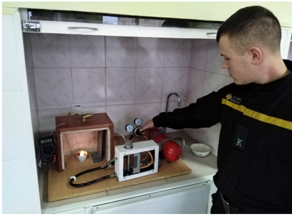
Fig. 4. Conducting experimental studies to determine the effect of gas exchange on the rate of extinguishing a fire with carbon dioxide
