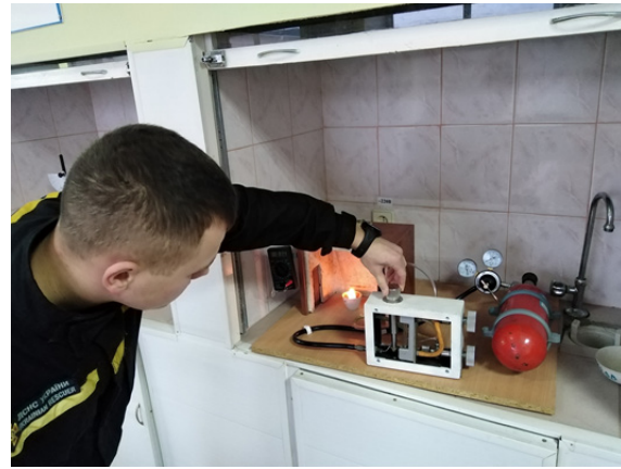
Fig. 4. Conducting experimental studies to determine the effect of gas exchange on the rate of extinguishing a fire with carbon dioxide
