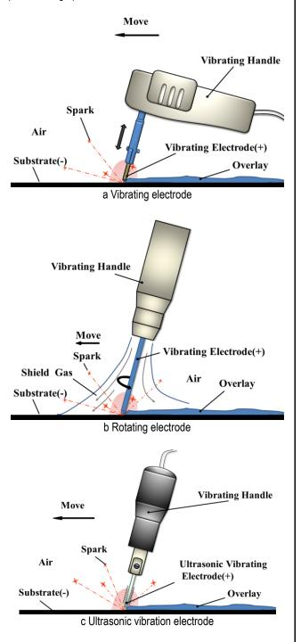
Fig.1 – Process diagram of electro spark deposition
