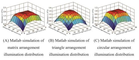
Fig. 6. Matlab simulation of illuminance distribution in different arrangement forms
