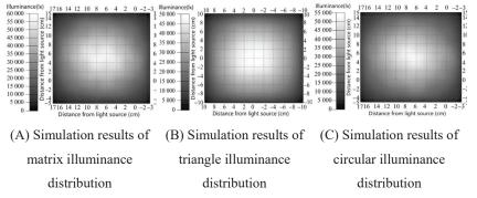
Fig. 5. Simulation results of illuminance distribution in different arrangement modes
